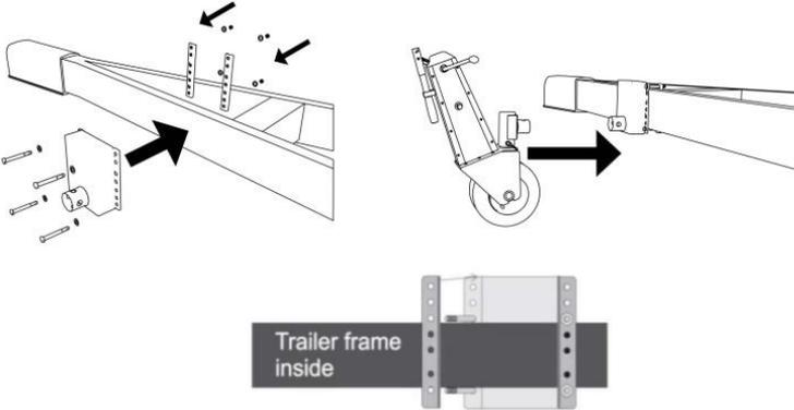
Place the connection point of the mounting joint into the mount bracket and fasten with the included stow/clevis pin. Lastly, set the cotter pin through the stow/clevis pin.
