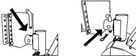
The Trailer Valet mounting bracket comes with a security bolt (part 7) that is an option to secure the device. This will add stability if needed, but may slow the process of attaching and detaching the unit from your trailer. If you choose to use it, the bolt slots through the back of the mounting bracket and threads into the mounting joint.
