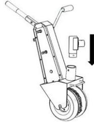
Place the mounting bracket and clamps onto the area of the frame you have designated and secure with the four bolts. **NOTE:** While it is recommended that the bracket is installed with the attachment point in the low position for stability reasons, the bracket can be flipped prior to install if the space is required.
